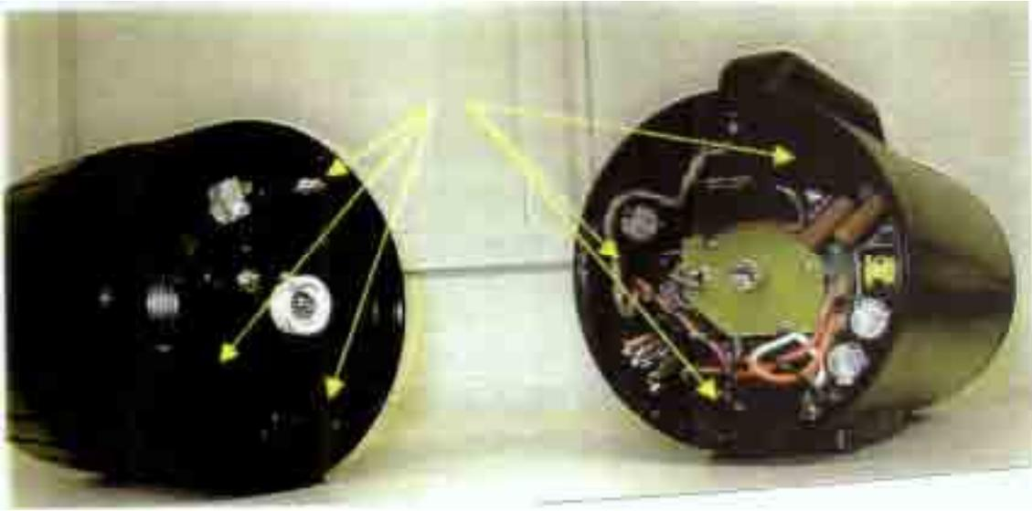
Figure 7.1 NightHunter After 30 inch Drop Test
