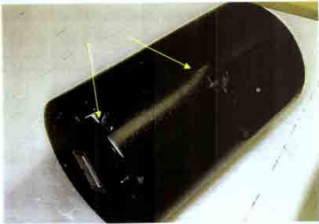
Figure 7.2 NightHunter Case After 30 inch Drop Test
